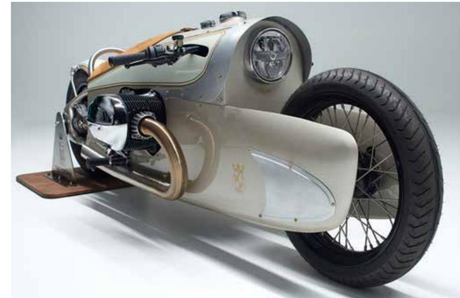
*Dirk Oehlerking and his team cut, bent and shaped the 2mm thick aluminum sheet to form the 8 liter fuel tank and body panels of the R18 The Crown. While the engine and rear suspension remain true to the original design, the two stainless steel exhaust manifolds are completely handcrafted.*
